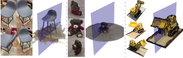
Figure A1. Generalization to object-centric scenes. We demonstrate accurate symmetry annotation on real (CO3D [31], left/center) and synthetic (NeRF-Synthetic [24], right) objects. We show sample input images and annotated symmetry planes overlaid on COLMAP MVS [34] point clouds.
